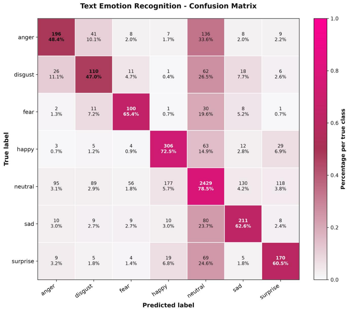
Figure 6.2: Confusion matrix of the text emotion recognition model on the test set
